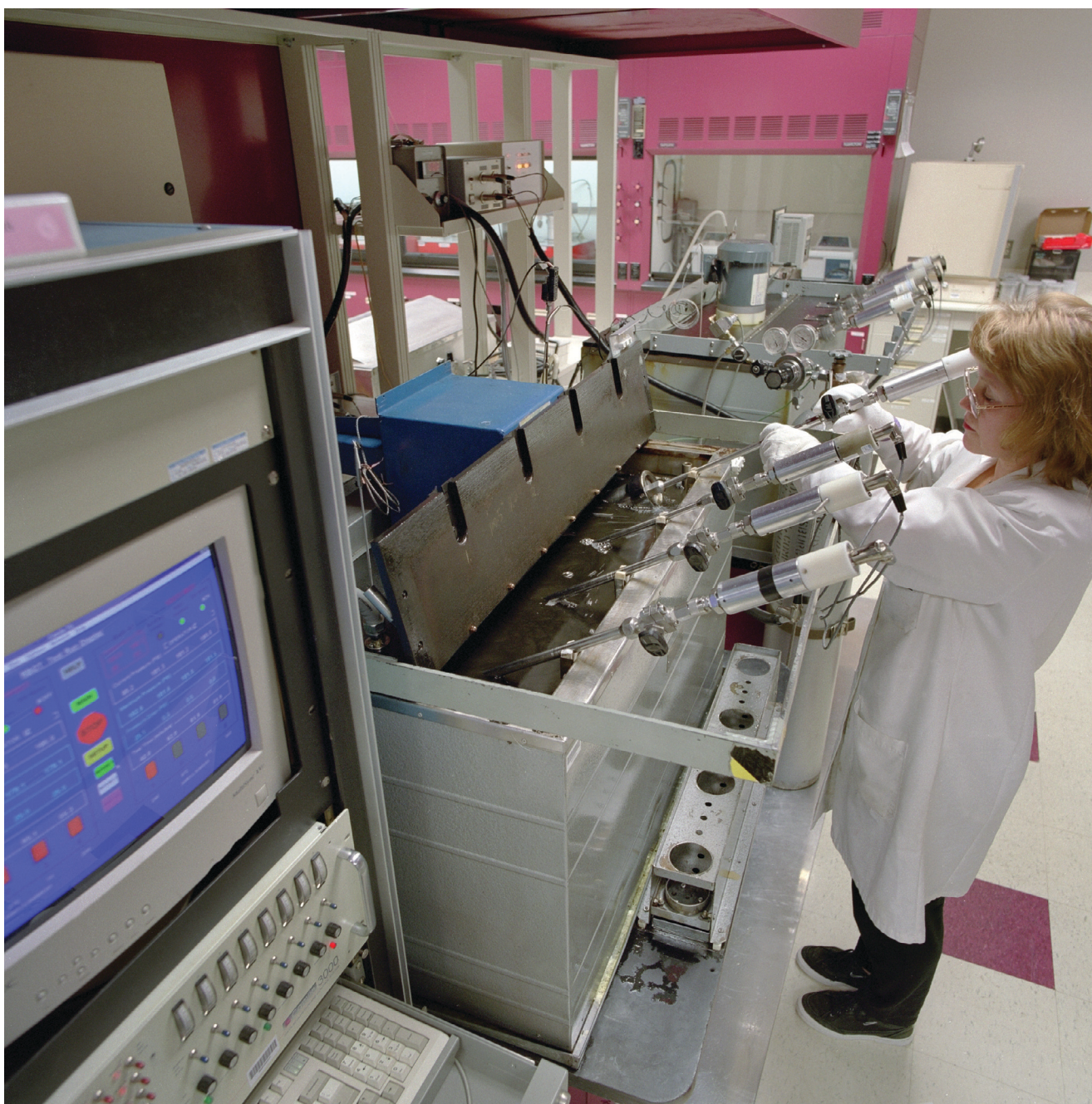
Figure 5 | The Rotary Bomb Oxidation Test is used to measure the effectiveness of antioxidants in lubricants under severe lab conditions. (Courtesy of The Lubrizol Corp.)
